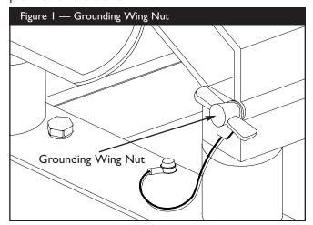
Generally, connecting a No. 12 AWG (American Wire Gauge) stranded copper wire to the grounding wing nut and to an earth—driven copper or brass grounding rod (electrode) provides adequate protection against electrical shock. However, local codes may vary widely. Consult with a local electrician for grounding requirements in your area. Be sure to keep the ground wire attached while you connect the electrode.
